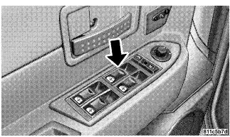
The control on the left front door has up-down switches that give you finger tip control of all four power windows. There is a single opening and closing switch on the passenger doors for passenger window control. The windows will operate only when the ignition switch is turned to the ON position and for ten minutes after the
